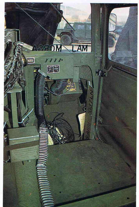
The co-drivers (or commanders) seat at right. The hoses are from the Hummer's heating system, one for the front occupant and one for the backseat passengers.
