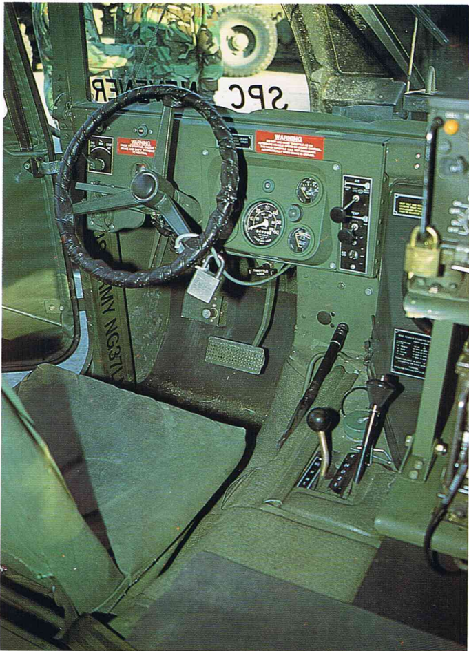
The drivers compartment with the gear levers and the handbrake next to the seat. When not in use, all 'HUMVEE's' have the cable and lock around the steering wheel to prevent theft. Unlike earlier days, every driver has his own vehicle and is therefore fully responsible for it's maintenance as well as it's state of performance.
