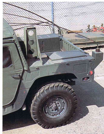
The aft cargo bay of the same vehicle. The typical antenna mount is one of the items in the VP kit. Note the way the antennas are tied down towards the front of the vehicle to avoid contact with the high voltage tension wires of railroad crossings.
