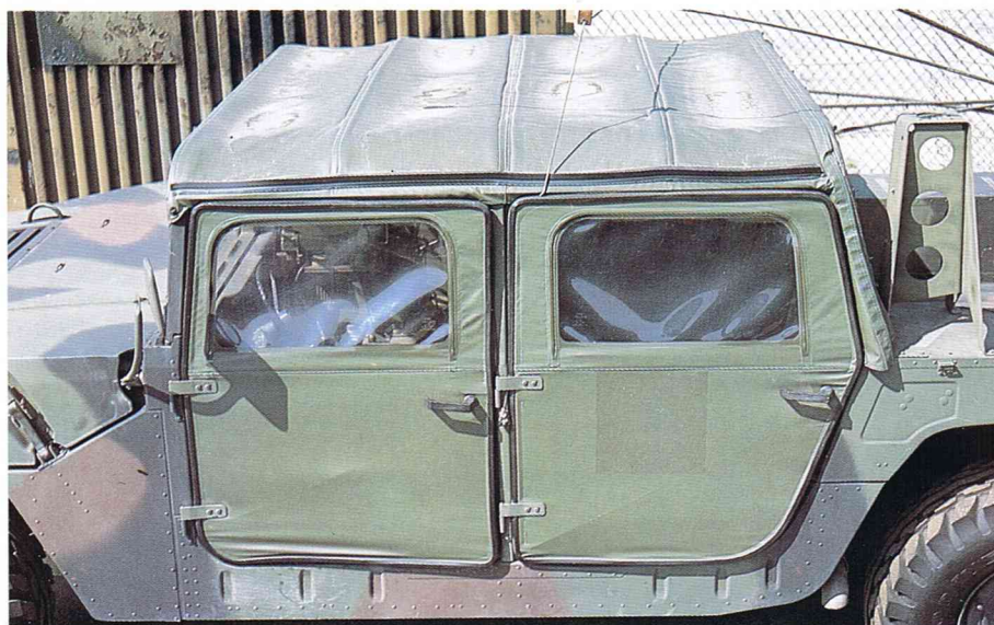
An excellent overall view of the canvas covered section of the M998 Command Vehicle, the subject of the first VP M998 Update Set. The exact size and shape of the soft plexiglass windows can be determined from the overall size of the vehicle and the doors. Note the outer frame, holding the canvas in place, is different in color. The purists will have to take care of the six indentations just below the doors which have been omitted on the Italeri kit.
