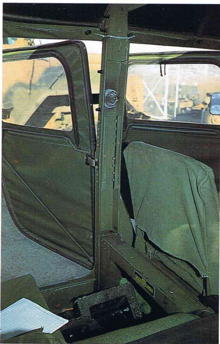
A view of the inside towards the left center frame bar and the back of the drivers seat. This angle clearly shows the inside detailing of the doors.
